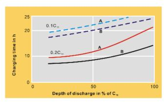
Re-charging time in relation to the initial charging current at 20  $^\circ\! C$  . Charge voltage:
