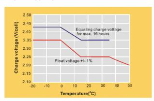
We recommend the volotage 2.25V for continuous charging. The charging voltage should be compensated to the curve under different ambinet temperature.
