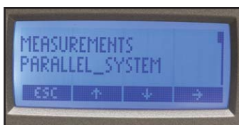
Access parallel system information
