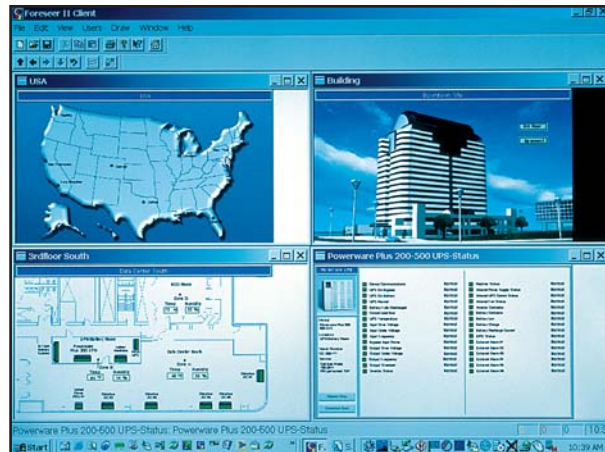
A configurable user interface displays critical data center information with FORESEER software.
